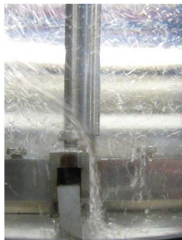
Fig. 10. Snapshot of \text{MgSO}_4 \cdot 7\text{H}_2\text{O} crystals scraped from the heat exchanger surface at 7 \times 10^{-1} s after starting up. In front and at the bottom of the scraper a triangular build-up of particles is formed.
