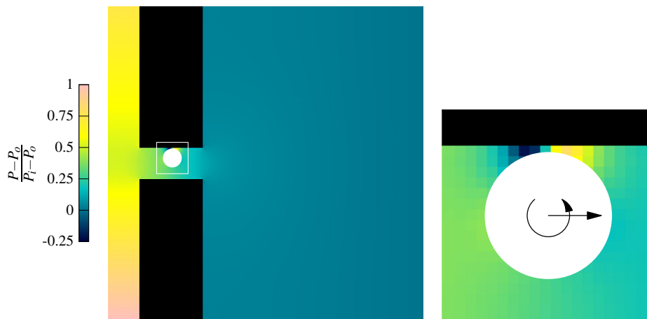
Fig. 14. Pressure field around the particle as it rotates and translates through the pinched segment during Run 7.
