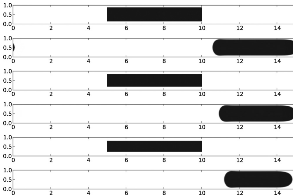
Fig. 3. Phase plots for different bubble thicknesses as H_{\text{eff}} = 12 , H_{\text{eff}} = 16 and H_{\text{eff}} = 20 . The grid for the simulation is 102 \times 1501 . The results are rescaled on N_y . The phase profiles were obtained after 2 \times 10^5 time steps. One can see that even if the system is initialized with different bubble volumes, the bubbles always relax to a shape where the film thickness is the same. For the given parameters ( Ca = 0.05 ) the interface thickness rescaled at the effective channel width H_{\text{eff}} is 0.0701, 0.0697, 0.0692 measured at the center of the bubble.
