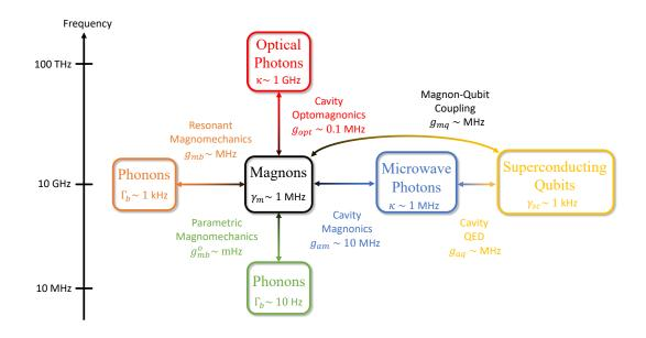
Figure 1.1: Characteristic frequency and the state-of-the-art decay rate and coupling rate for each hybrid magnonic system. See the main text for examples of each form of coupling. Modified from Ref. [13]
