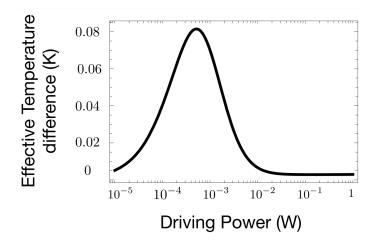
Figure 8.4: Difference between the effective temperature given by the full formula Eqn. 8.29 and the improved approximation Eqn. 8.34. For this plot we have used the experimental parameters and driving scheme corresponding to the results of Fig. 9.8, and the bath temperature is  $T_{\text{Bath}} = 295$  K.
