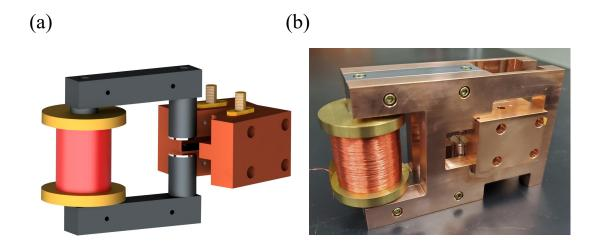
Figure C.1: Tunable magnet. (a) Rendered schematic of the tunable magnet. Pure iron yoke with a pair of disk-shaped neodymium magnets provides the static bias field. A  $\sim 10^4$  turn solenoid provides tunability about the bias field set point. (b) Photograph of the tunable magnet.
