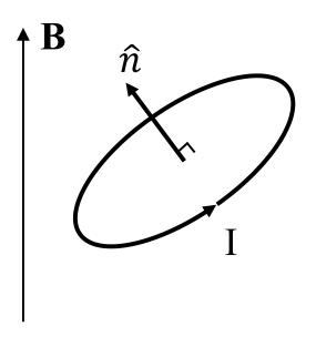
Figure 2.1: Loop of current in a static magnetic field.
