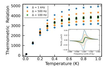
Figure 8.7: Thermometric relation for different finite detunings of the MW drive. As the detuning increases  $S_{0,\pi/2}[\omega]$  is contaminated with a contribution from the phonon thermal occupancy. Inset shows  $\operatorname{Re}\{S_{0,\pi/2}[\omega]\}$  for the same detunings. Diamond markers and dashed lines represent negative detunings.
