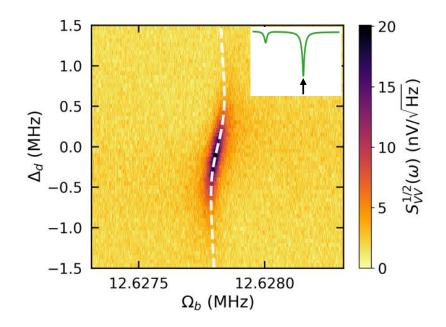
Figure 9.6: Magnon spring effect. Power spectral density of the mechanical motion within a partial pressure of helium gas and a constant probe power of 0.13 mW. The microwave drive was tuned to the normal mode shown in the inset. The white curve is the theoretical prediction for the magnon-spring effect, see chapter 8, the only fit parameter was the intrinsic mechanical frequency.
