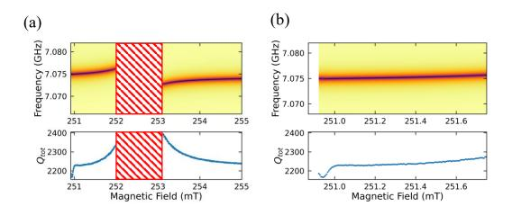
Figure 7.3: (a) Top: Measured normal mode spectrum as a function of the static magnetic field. Bottom: Total quality factor of the 'photon-like' microwave resonance as a function of the static magnetic field. At  $\sim 251$  mT a sharp dip can be observed in the quality factor due to weak coupling to a higher-order magnon mode. (b) Zoom of (a) near the weak magnon-photon coupling.
