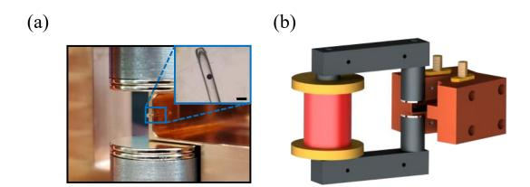
Figure 7.1: (a) Photograph of half of the microwave cavity, made from oxygen-free copper. The YIG sphere is placed – free to move – within a glass capillary, inner dimension of approximately 300 microns. Inset: Optical micrograph of the YIG sphere inside of the glass capillary. The scale bar is 500 microns. (b) A set of permanent neodymium magnets attached to a pure iron yoke provide the bias magnetic field, a solenoid allows the bias field to be varied dynamically.
