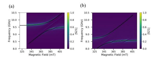
Figure 7.5: (a) Normalized transmission spectrum  $(S_{21}(\omega)))$  of the tunable YIG microwave cavity system as a function of the external magnetic field. The helium reservoir pressure was set to 2 bar. The solid black line is a fit to the coupled magnon-photon system described by Eqn. 7.2. (b) Normalized transmission spectrum  $(S_{21}(\omega)))$ , for a helium reservoir pressure set to 6 bar. Note, that both figures have been plotted on the same axes.
