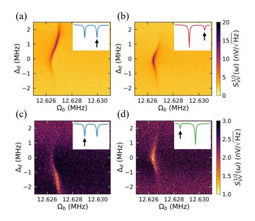
Figure 9.9: Magnon Heating. (a-d) Mechanical power spectral density. Detuning is relative to the specific mode shown within the inset. Plots (a) and (c) the probe power is held constant at 0.54 mW. Plots (b) and (d) the probe power is held constant at 0.27 mW. All data presented was obtained with the experimental setup in atmospheric conditions.
