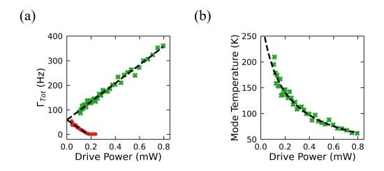
Figure 9.8: Magnomechanical cooling. (a) Mechanical linewidth as a function of drive power in vacuum. Red circles demonstrate magnomechanical anti-damping and includes the data from Fig. 9.5(b), green crosses demonstrate magnomechanical damping and includes the data from Fig. 9.5(c). (b) Effective mode temperature of the mechanical mode determined from Eqn. 9.4.
