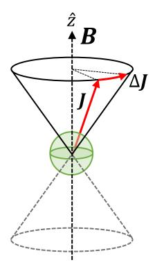
Figure 2.2: Illustration of the Larmor precession. Over a small time interval  $\Delta t$ , the angular momentum changes by a small amount  $\Delta \mathbf{J}$ , revolving around the z axis with a frequency  $\omega_L$ .
