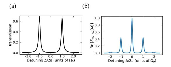
Figure 8.8: (a) Transmission spectrum of a strongly coupled magnon-photon system showing hybridized magnon-photon modes separated by  $2g_{\rm am}$ . b) Phase-phase correlation function for  $\omega = \Omega_{\rm b}$ . The magnon-photon coupling rate was set to equal the phonon frequency,  $g_{\rm am} = \Omega_{\rm b}$ , resulting in a peak in the correlation function at zero detuning,  $\Delta_{\rm a} = 0$ , corresponding to the measurement prescribed in the text.
