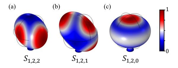
Figure 4.2: Simulated displacement profile  $\mathbf{u}(\mathbf{r})$  of a YIG sphere attached to a small supporting post.  $S_{1,l,m}$  defines the spherical modes with radial mode number 1, angular mode number l, and azimuthal mode number m.
