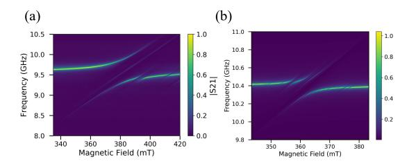
Figure F.1: (a) Experimentally measured transmission coefficient (b) COMSOL simulation demonstrating strong magnon-photon coupling.
