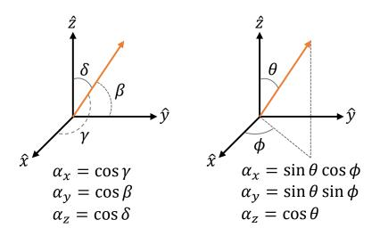
Figure 6.1: Definition of the directional cosines in terms of angles from the principle Cartesian axis, as well as using standard spherical coordinates.
