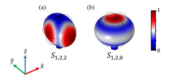
Figure 6.2: Simulated displacement profile  $\mathbf{u}(\mathbf{r})$  of a YIG sphere attached to a small supporting post.  $S_{1,l,m}$  defines the spherical modes with radial mode number 1, angular mode number l, and azimuthal mode number m.
