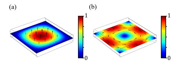
Figure 3.2: FEM simulation of the  $TE_{101}$  mode of a rectangular microwave resonator with dimensions  $30 \times 30 \times 6 \text{ mm}^3$ . (a) Normalized electric field distribution. (b) Normalized magnetic field distribution.
