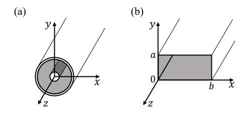
Figure 3.1: Schematic of metallic waveguides. (a) Cross-section of a coaxial waveguide. (b) Cross-section of a rectangular waveguide.
