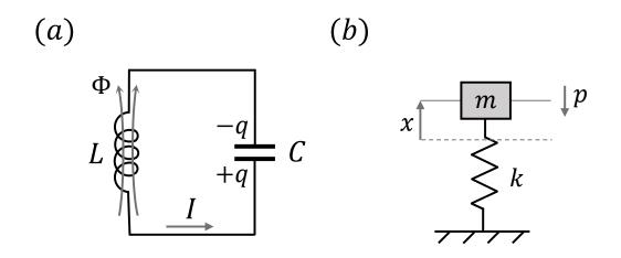
Figure 3.4: (a) Schematic of an LC resonator. (b) Schematic of a mass-on-a-spring simple harmonic oscillator.
