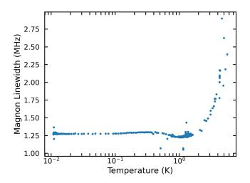
Figure E.1: Temperature Dependence of Magnon Linewidth. A minimum in the magnon linewidth exists at approximately 1K; a slight increase is observed below this temperature and has been attributed to two-level system relaxation; see Ref. [17] for a full discussion.
