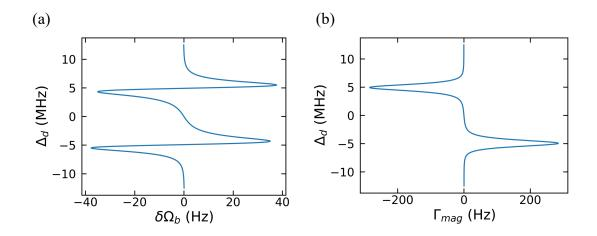
Figure 8.2: (a) Magnon-Spring effect predicted from Eqn. 8.19. (b) Magnomechanical damping rate predicted from Eqn. 8.19. Parameters are listed in the main text.
