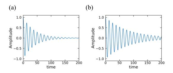
Figure 4.3: Normalized displacement amplitude x(t) of a damped harmonic oscillator described by Eqn. 4.28, where we have set  $\theta_0 = 0$ , and the oscillation frequency  $\omega = 0.5$  rad/s. Both are plotted in arbitrary units. (a) Decay rate  $\Gamma = 0.1\omega$ . (b) Decay rate  $\Gamma = 0.05\omega$ .
