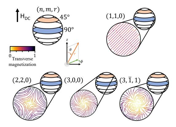
Figure 2.3: Spatial magnetization of specific magnetostatic modes in a YIG sphere orthogonal to the static magnetic field.
