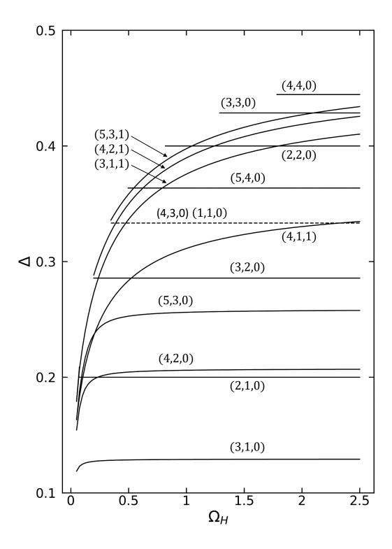
Figure 2.4: Magnetostatic mode frequency for different Walker modes. Here we have plotted the dispersion using normalized units  $\Omega_H = \frac{H_i}{M} = \frac{H_0 - M_S/3}{M_S}$  and  $\Delta = \Omega_H - \Omega$ . Adapted from Ref. [68].
