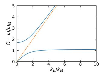
Figure A.1: Magnon dispersion relationship  $k_b$  for propagation perpendicular to the applied field. The wavenumber is normalized by  $k_M = \omega_M \sqrt{\mu_0 \epsilon}$ , and we further used  $\omega_0 = \omega_M$ . The dashed line corresponds to the dispersion relationship for  $k = k_a = k_0$ .
