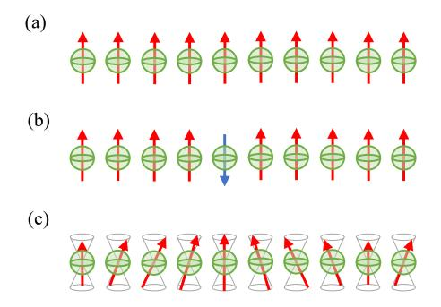
Figure 2.5: Schematic representation of a one-dimensional spinwave excitation, whose quanta of excitation is the magnon. (a) Spin-polarized ferromagnetic ground state, (b) Single spin-flip state, (c) the spin-wave state.
