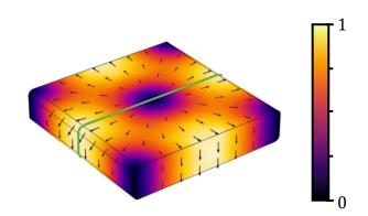
Figure 3.3: Normalized surface current distribution for the  $TE_{101}$  mode of a rectangular microwave resonator. The green line indicates the location of the seam separating the two halves of the resonator.
