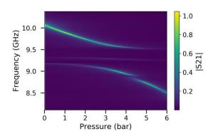
Figure 7.6: Normalized transmission spectrum  $(S_{21}(\omega))$  of the tunable YIG microwave cavity system as a function of helium reservoir pressure. The magnetic field was held constant at ~ 380 mT.
