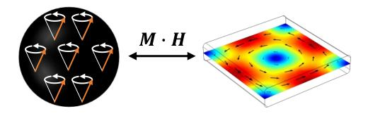
Figure 5.1: Schematic of magnon-photon coupling. Spins within the YIG sphere couple via the Zeeman interaction to the time-varying microwave cavity magnetic field. This schematic is not to scale, the YIG sphere is on the order of 250  $\mu$ m in diameter, and the microwave cavity has dimensions  $30 \times 30 \times 6$  mm.
