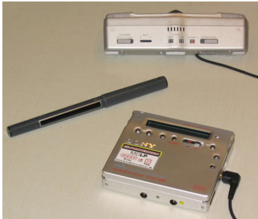
Mini-disc recorder and desktop digital microphone – shown with a pen for size comparison.
