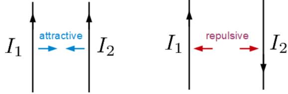
The force per length between two wires at a distance  $R$  is
