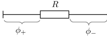
Hence the potential must change from  $\phi_+$  on the left connection (“lead”) of the resistor  $R$  to  $\phi_-$  on the right connection point by the voltage drop
