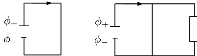
They contain a wire that connects two points of supposedly different potential  $\phi_+ \neq \phi_-$ . This leads to the flow of an extremely large current that heats up the wire (Joule heating) and typically destroys the circuit.
