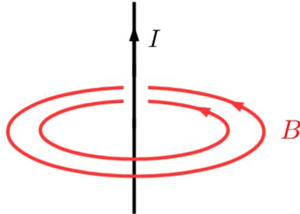
The  $B$ -field points into the azimuthal direction and forms a "right-hand-system" with  $I$ , where the thumb points in the direction of  $I$  and the fingers curl into the direction of  $B$ . Consider two wires carrying the same currents  $I$  at a distance  $R$  apart. One at  $x = y = 0$  along the z-direction, one at  $x = R, y = 0$  along
