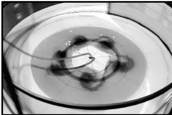
FIGURE 4. Perspective view of three experiments characterized by parameters \Omega (the rotation rate) and \Delta\rho (the density difference between the injected and ambient fluid), as indicated. The depth of the ambient ( H_T = 15 \text{ cm} ) and the fluid injection time ( T_{inj} = 30 \text{ s} ) is the same in all three cases. Snapshots are taken approximately one minute into the experiment, 30 s after fluid is no longer being injected.
