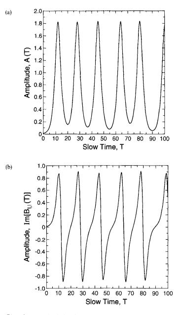
Figure 7a, b Plot of temporal solution for (a) A(T) and (b)  $\text{Im}[B_{1,1}(T)]$  for the 4 equation set (5.38) where k = 0.5, l = 0.866, and  $A_0 = 0.01$ .
