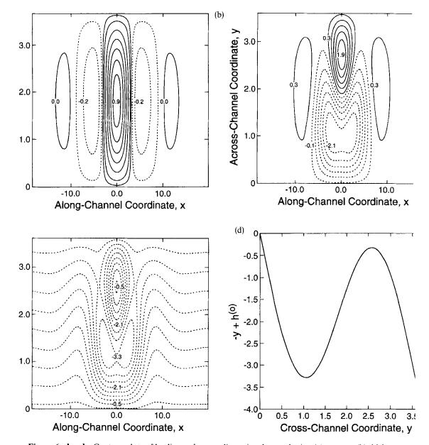
Figure 6a, b,c, d Contour plots of leading order non-dimensional perturbation (a) pressure (b) thickness and (c) leading order variable part of the total current height scaled by  $\varepsilon^{-2}$  where k = 0.5, l = 0.866, and  $A_0 = 0.5$ . The contour intervals in (a), (b) and (c) are approximately  $\pm 0.15$ ,  $\pm 0.4$  and  $\pm 0.4$ , respectively. Figure 6d depicts a section along x = 0.0 from Figure 6c. Note the distinct positive anomaly centered at approximately  $y \simeq 2.5$ .
