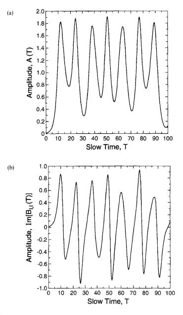
Figure 8a, b Plot of temporal solution for (a) A(T) and (b)  $\text{Im}[B_{1,1}(T)]$  for the 12 equation set truncated at  $\alpha_6$ ,  $B_{2,4}$  for even gravity current modes and  $B_{3,5}$  for odd gravity current modes. Parameters are the same as in Figures 7a, b.
