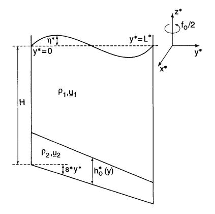
Figure 1 Geometry of the channel two-layer model.
