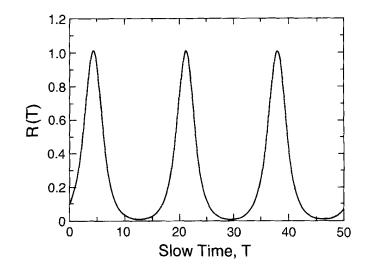
Figure 3 Plot of non-dimensional perturbation pressure amplitude R(T) versus time T, where k = l = 1.0 (i. e. N = 1.0),  $\varepsilon = 0.1$  and where  $\eta = \varepsilon \eta_0 + O(\varepsilon^2)$ .
