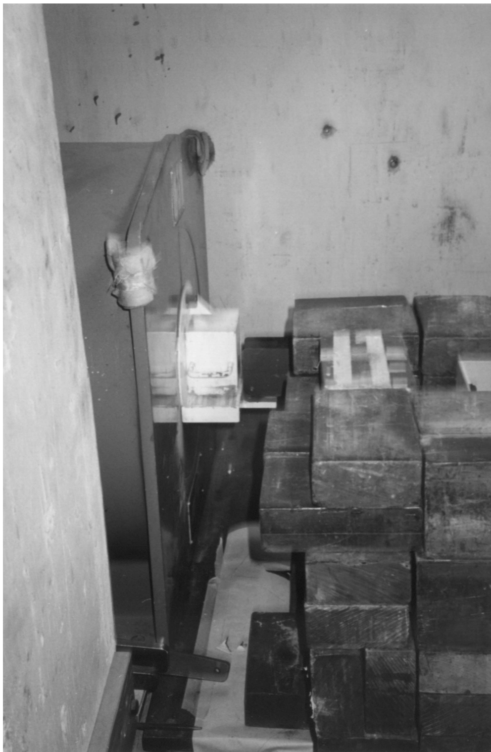
Figure 5.3: Photograph of ^{60}\text{Co} facility showing the containment tank on the left and the lead sample enclosure on the right.
