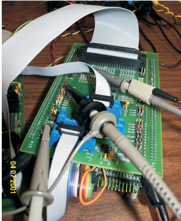
Figure E.1: Photograph of the monitor board used for the DMILL ASIC and XC2S150E tests. In the photograph probes are attached to the board for monitoring signals during one of the tests.
