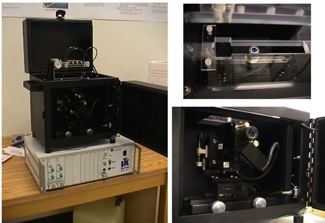
Figure C.2: The \mu TK Apparatus. The \mu TK is a platform for electrokinetic microfluidics. The apparatus consists of an high voltage power supply that supplies a (software) set voltage to platinum electrodes which are located on a lowerable assembly. A microchip is set in a machined plexiglas holder below the electrode assembly, below which a 40X microscope objective is positioned allowing imaging of microchannels. The optics module is an epiluminescent confocal microscope allowing fluorescent excitation (images courtesy of MicroLyne Inc.).
