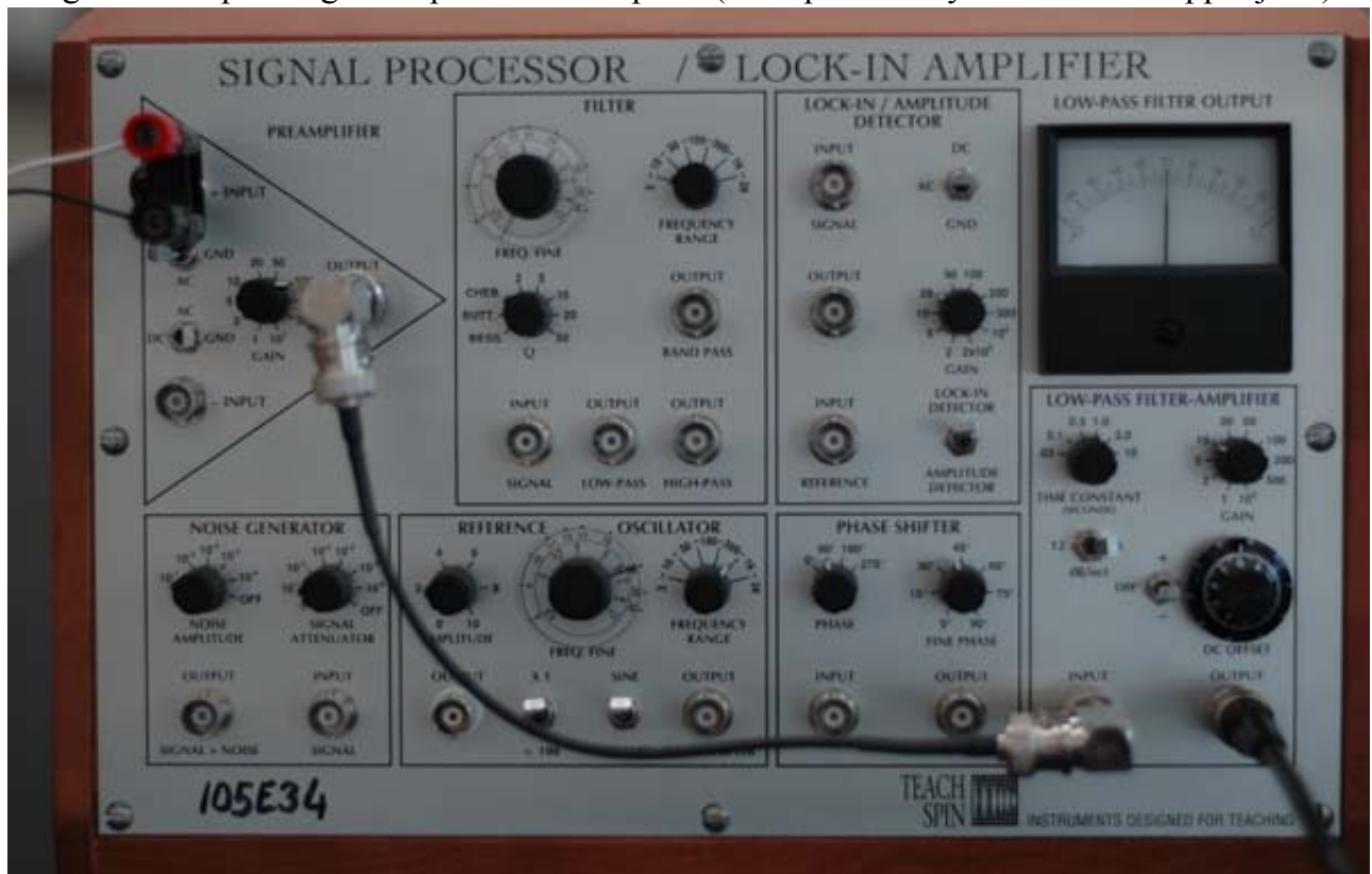
Fig 3: the signal processor front panel, with output of preamp connected to input of low-pass filter-amplifier in improvised fashion, using a too-short coax.
