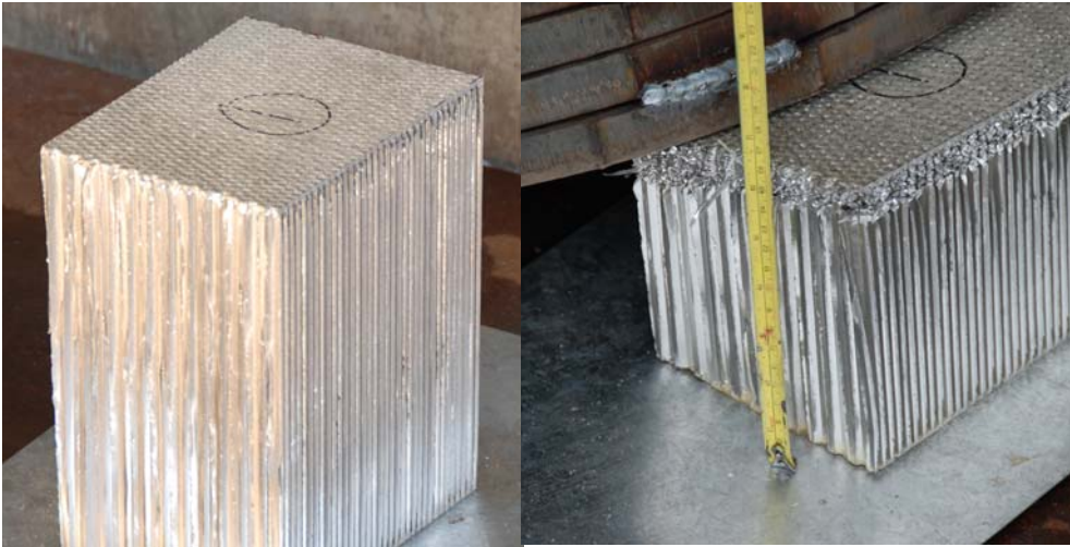
Before and after of an Impact Attenuator Test Crush.
