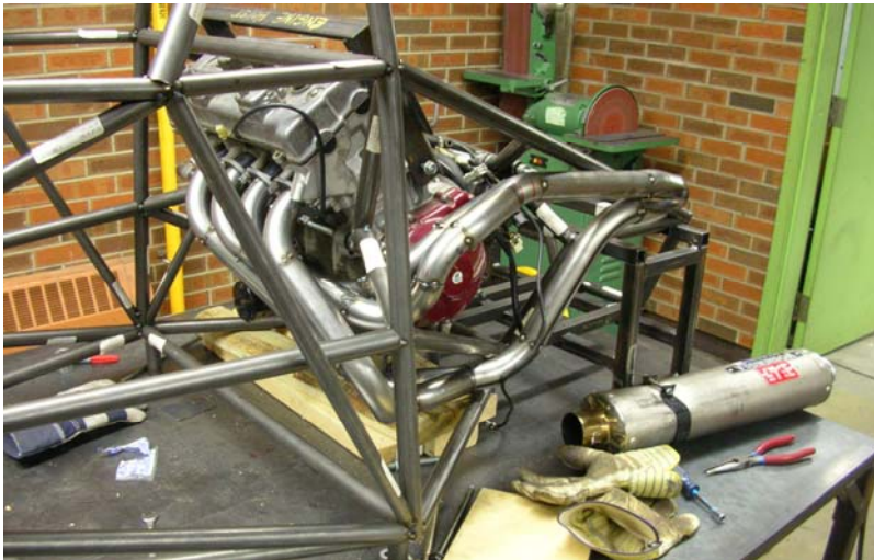
Exhaust and engine being fitted within the chassis.
