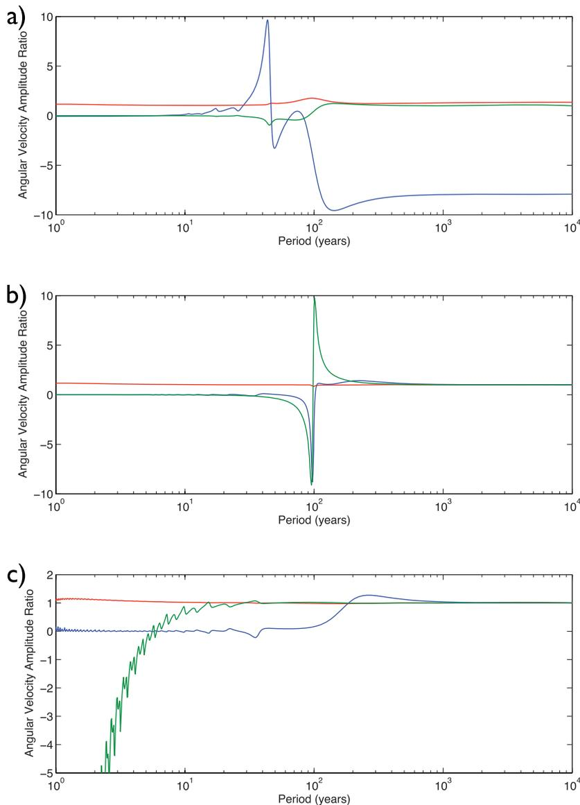
**Figure 1.** Angular velocities relative to that of the inner core for a forcing applied to the (a) tangent cylinder (b) inner core and (c) mantle. All panels show the velocities of the fluid inside the tangent cylinder (red lines), the fluid outside the tangent cylinder (blue lines) and the mantle (green lines). The viscous relaxation time of the inner core is  $\tau = 1000$  yr, all other parameters are as given in Table 1.
