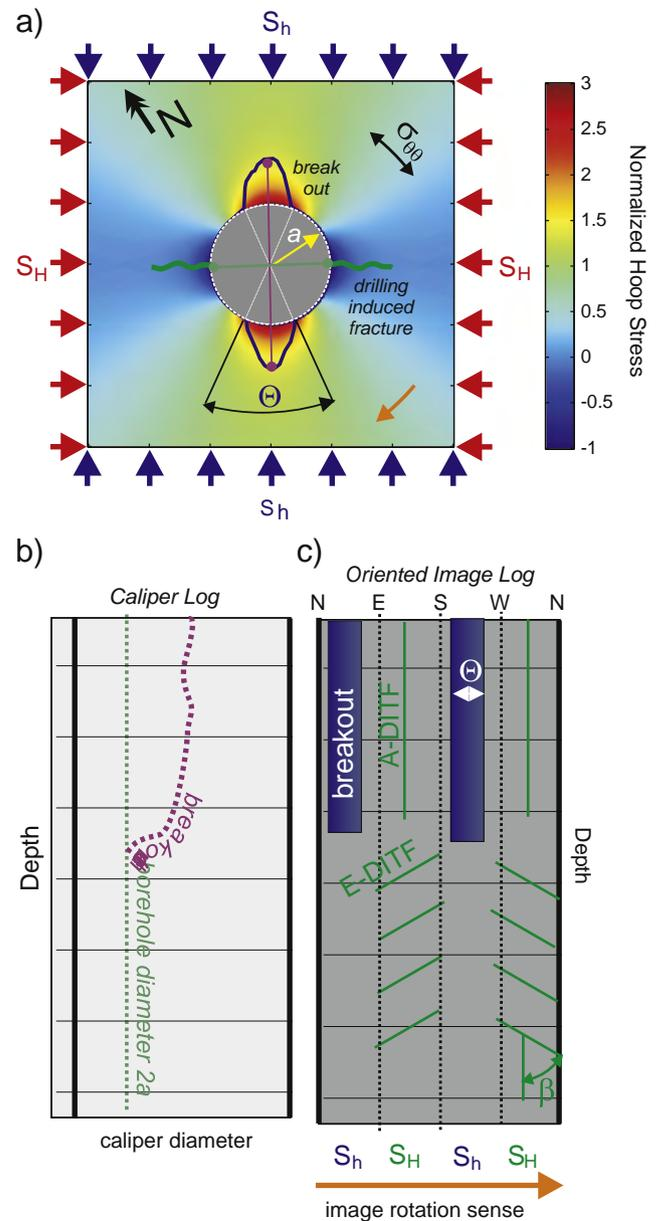
**Fig. 19.** Cartoons of a) stress induced borehole deformation with the corresponding b) oriented caliper log (e.g., dipmeter), and c) oriented image log. Both axial (A-DITF) and en-echelon (E-DITF) drilling induced tensile fractures (green) and borehole breakouts (blue) that are parallel and perpendicular to the  $S_H$  spring-line, respectively.
