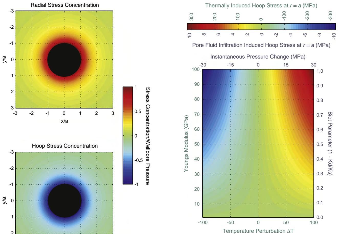
Fig. 6. Stress concentrations, normalized with respect to the wellbore fluid pressure, at the borehole wall resulting from the fluid pressures for the radial stress  $\sigma_{rr}$  (top panel) and the azimuthal hoop stress  $\sigma_{\theta\theta}$  (bottom panel).
