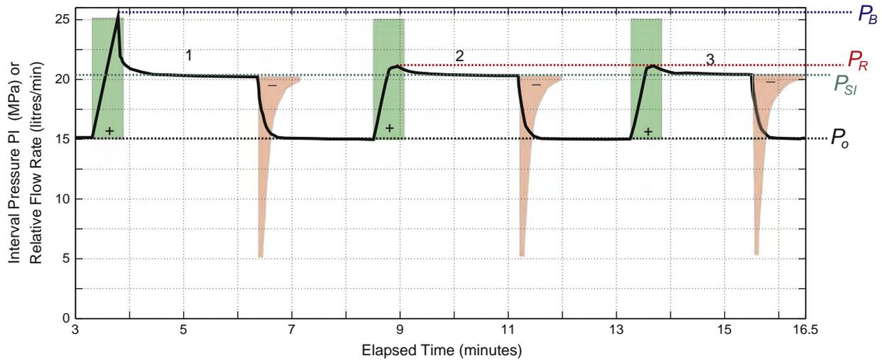
**Fig. 15.** Illustration of a typical hydraulic fracturing (micro-frac) stress measurement. Heavy black line represents the pressure recorded within the interval. Green and red shaded areas represent flow rates into or out of the interval, respectively.
