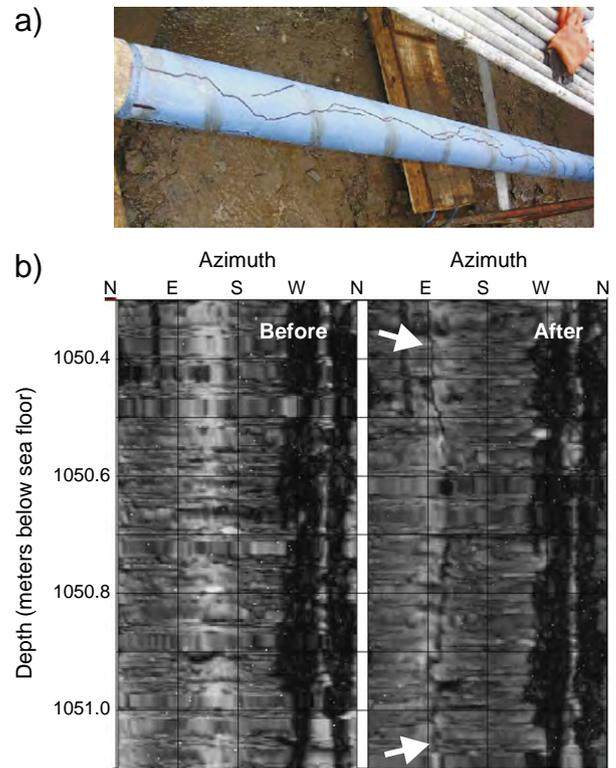
**Fig. 16.** a) Photograph of an impression packer after removal from the borehole displaying the trace of the induced fracture on the borehole wall. b) Example of borehole televiewer images taken before and after a hydraulic fracture test at a depth of 1050.7 m below the sea floor as part of the ANDRILL South McMurdo Sound drill hole. The induced fracture highlighted between the two white arrows suggests that  $S_H$  is directed ESE.
