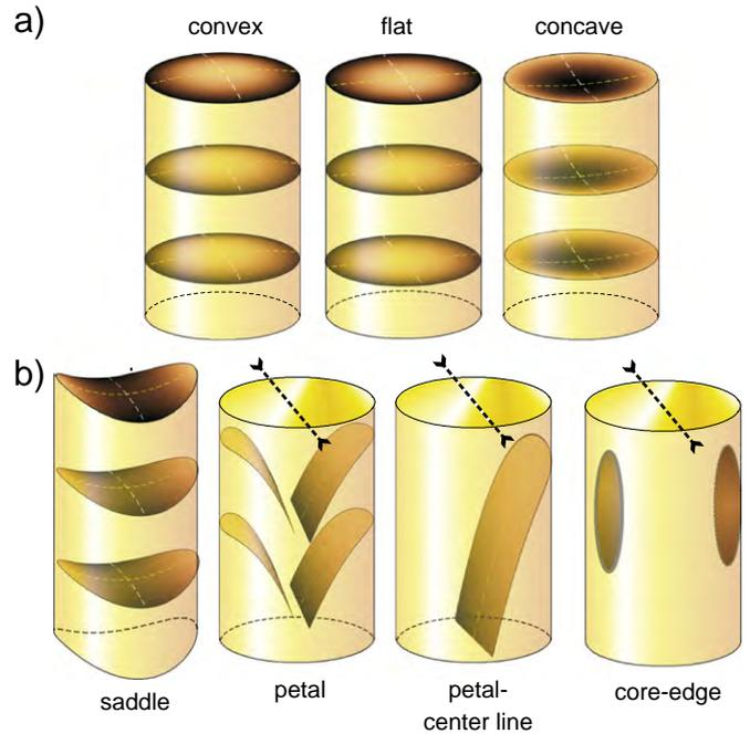
**Fig. 23.** Classification of differing types of drilling induced core fractures from a vertical bore-hole. a) Disk fractures formed under a uniform state of horizontal stress. b) Saddle-shaped, petal, and core edge fractures formed under an anisotropic state of stress perpendicular to the borehole axis. The strike of these fractures (shown by dashed lines) indicates the direction of  $\sigma_H$ .
