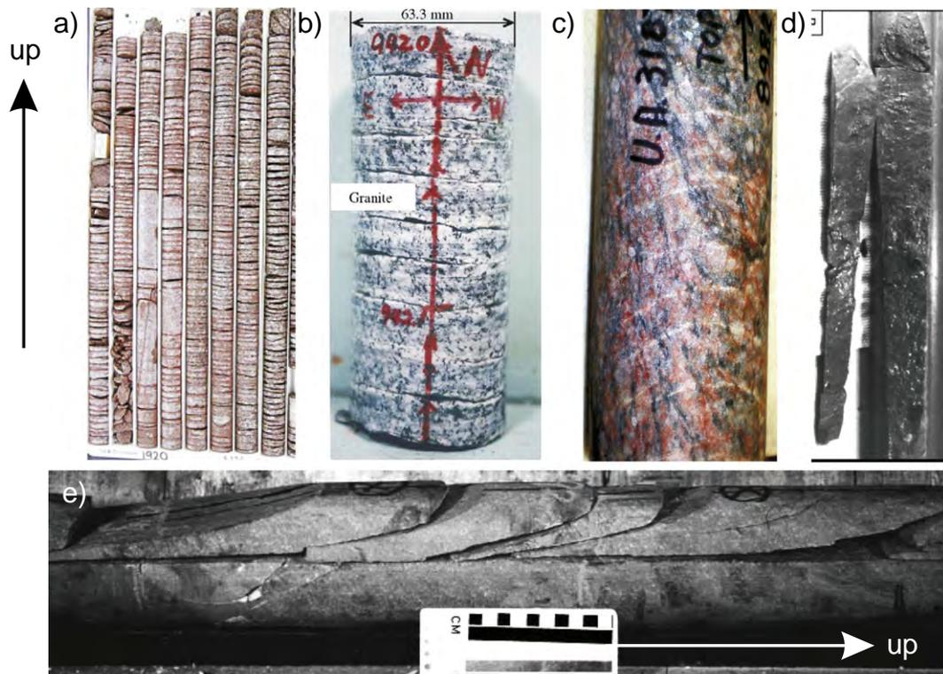
**Fig. 21.** Examples of drilling induced core fracture phenomena. a) Series of flat core disks along length of core. b) Series of uniformly spaced concave saddle shaped disks from a depth of 942 m from a vertical borehole at Sakuma, Shizuoka prefecture, Japan. c) Petal fractures in metamorphic rock from the Canadian shield in Alberta. d) Example of core-edge fractures. e) Series of petal-centerline fractures in West Texas limestone core.
