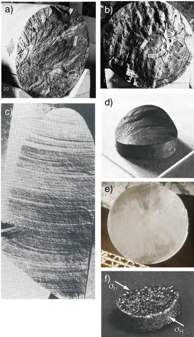
**Fig. 22.** Examples of drilling induced core fracture surfaces showing tensile nature. a) Disk fracture initiating from core edge, b) disk fracture initiating from core axis, c) petal-centerline fracture initiating at core edge, d) convex saddle shaped core disk, e) weakly concave disk fracture with fracture initiation point near center of core in brittle shale, f) concave saddle shaped disk produced in laboratory experiments on Westerly granite.
