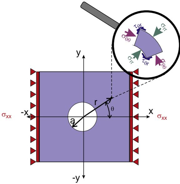
**Fig. 3.** Geometry of Kirsch's (1898) solution for the stress concentrations around a circular hole is a plate that is subject to a uniaxial stress  $\sigma_{xx}$ . Cylindrical element at location  $(r, \theta)$  is magnified to show the cylindrical stresses acting on it.
