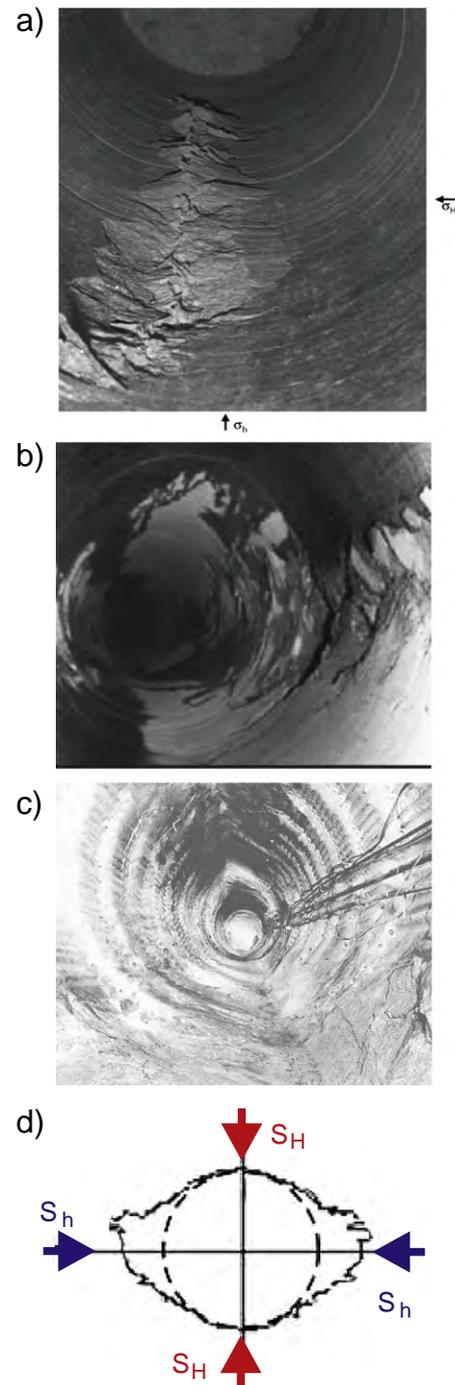
**Fig. 17.** Photographs of borehole breakouts. a) Incipient extensile buckles on the floor of a borehole drilled in crystalline rock. b) Down-hole borehole breakouts. c) Extensive breakout formation around a circular tunnel excavated in granite. d) Cross-section shape of a breakout in a Hawaiian basalt flow.
