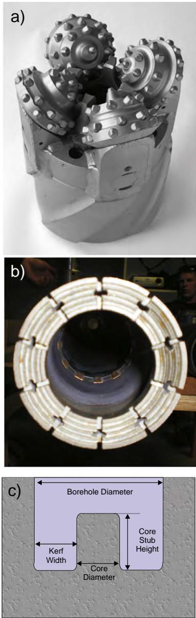
**Fig. 24.** Types of coring bits. a) Rotary tri-cone core bit produces 58.7 mm diameter core, b) typical PQ-dimension diamond impregnated coring bit with 85.09 mm diameter core, c) side view through the borehole bottom showing the core stub. Panel a is a photo from <http://www-odp.tamu.edu/publications/tnotes/tn31/title.htm> with permission for use granted from ODP Publication Services. Panel b is a photo courtesy of D.R. Schmitt.
