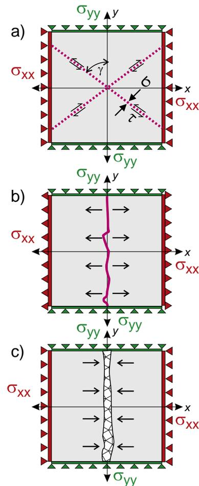
**Fig. 11.** Illustration of the modes of rock failure. a) Shear failure under compressive stress state  $\sigma_{xx} > \sigma_{yy}$ , b) tensile failure produced by pure tension  $\sigma_{xx}$ , c) compaction band collapsing parallel to  $\sigma_{xx} > \sigma_{yy}$ .
