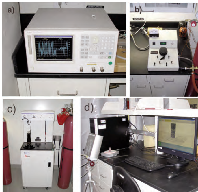
Figure 6. Various laboratory instruments. a) 10 MHz to 3 GHz dielectric impedance measurement system, b) He pycnometer, c) Hg porosimeter, d) 3D image scanner.
