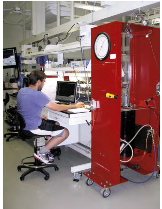
Figure 1. 'Red' pressure vessel with capacity to 300 MPa total pressure with undergraduate student Brendan Snow making P and S wave measurements on shocked materials.
