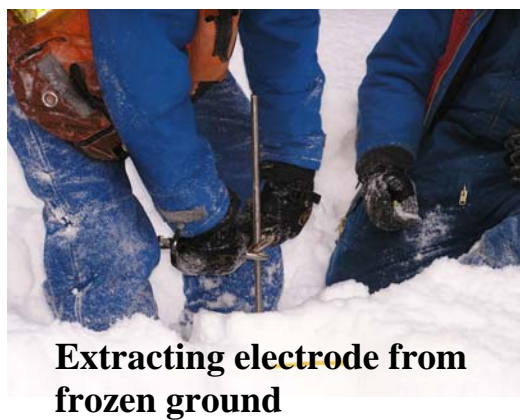
Figure 5.2: ERT field photographs, author standing of right. Cold weather conditions made working conditions difficult but provided good coupling of electrodes with the ground. Difficult to pull electrode due to hard snow (left bottom panel). Electrical resistivity tomography instrument (right bottom panel).
