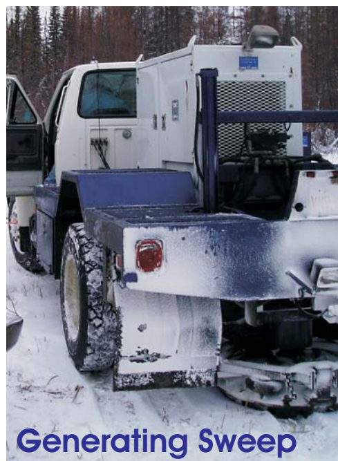
Figure 4.9: U of Alberta vibrator working in the field. Photographs courtesy of Marek Welz.
