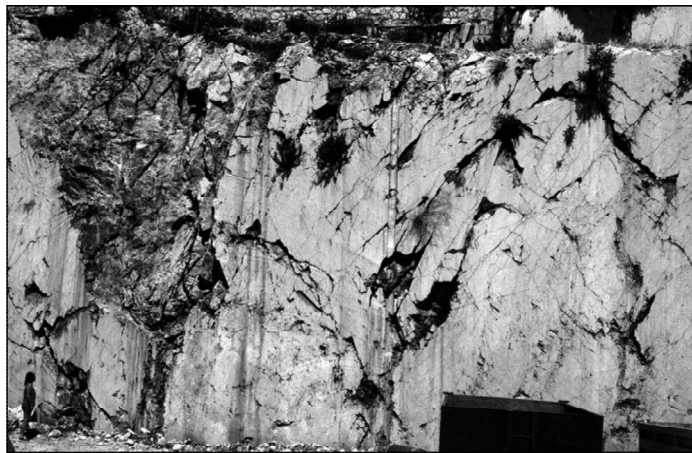
Figure 2.13: Cutaway limestone face in a construction area in Sicily exhibiting a buried sinkhole on the left and dissolution fissures on the right [reproduced from Walsham and Fookes, 2003 ]. Person is shown on bottom left corner for scale.
