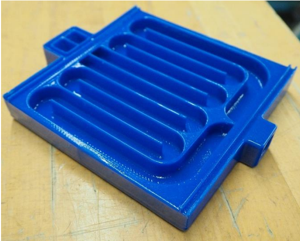
Figure 4.35 Image of an ABS part that has been acetone vapor smoothed but not heated.
