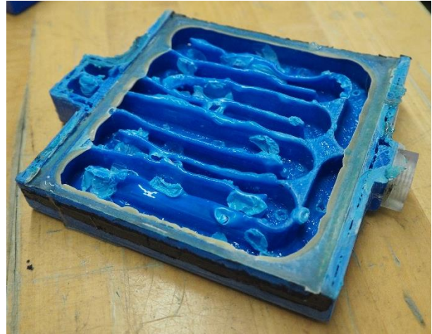
Figure 4.36 Image on an ABS part that has been acetone vapor smoothed and then heated up to 95 °C.
