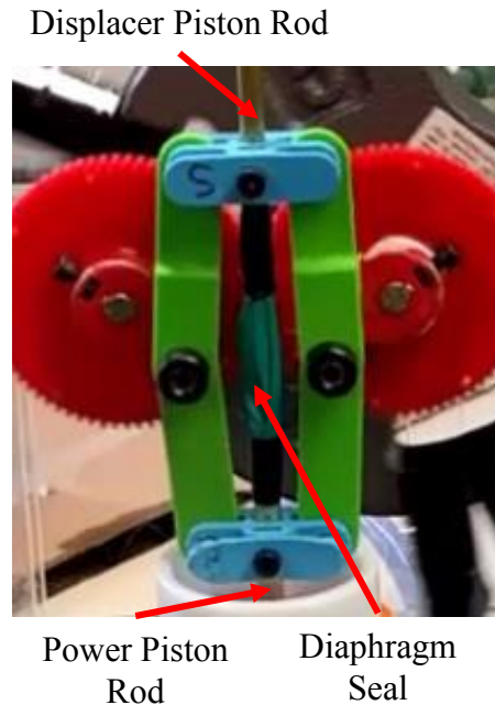
Figure 4.7 Image of the rubber diaphragm seal used for the displacer piston rod power piston rod interface.
