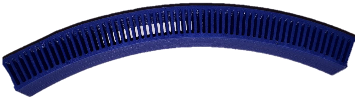
Figure 4.47 Image of a section of the slotted regenerator used by the EP-1.
