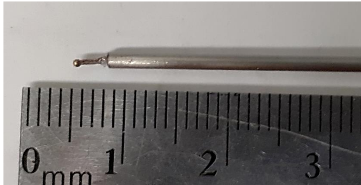
Figure 3.3 Image showing the size of the sensing mass for the Type-T thermocouples used.
