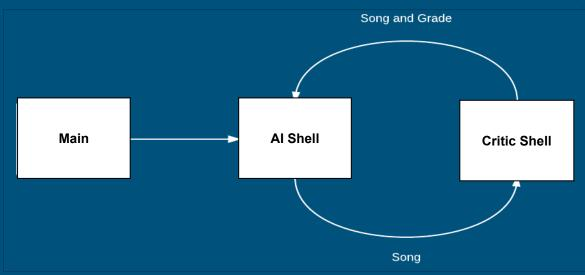
Main: accepts random seed; contains running loop; interacts with DE2 via ethernet, AI Shell: creates songs based on input and prior songs, Critic Shell: grades songs
