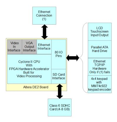
The first additional feature is the ability to store past data that was processed by the CPU. This would require first a storage medium and also a method to compress the frame data into video files that can be stored. The storage medium that we want to use is the SD card interface with the onboard SD interface. For compression, we will try to utilize the MP4 compression algorithm to store the video.[8]
