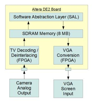
The system starts by receiving an NTSC video feed from the security camera through the video in interface. This is interfaced on the DE2 using the onboard video-in port with the onboard ADV7181B chip. The NTSC standard supports a maximum of 30 frames per second which is the targeted rate that the Cyclone II CPU will be able to process the data. The video feed will then be processed, which will be
