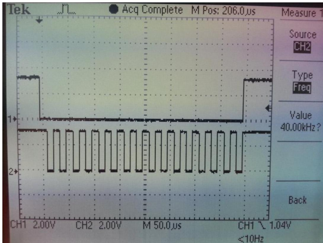
Channel one displays A\_en, while channel two display TxA. Notice that the frequency reading from the oscilloscope displays the desired frequency. Probing the B\_en, and TxB pins while A\_en is being asserted also displays both B\_en and TxB staying at logic 1 while A is transmitting, satisfying our needs.
