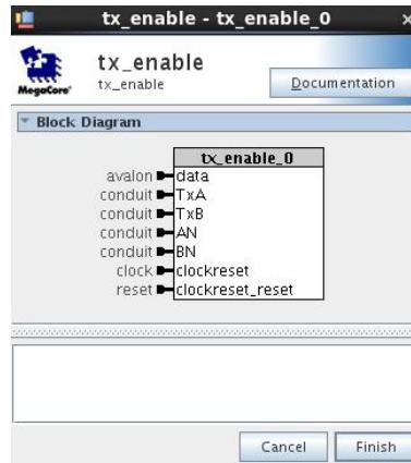
Note that the conduit signals are the signals that will be generated in your *projectname\_system.vhd* file. Your top level entity will require port mapping of these four signals to GPIO pins.
