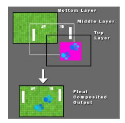
Each of these hardware features involve a storage cost in the SDRAM. The overall function of the SDRAM in the system is to provide a scratch space for compositing frames. These frames, when composited, are sent to the SRAM when timing allows, as previously described.
