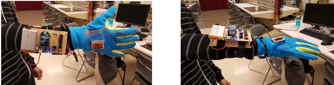
The design of the project can be split into two modules. The glove module is composed of all the hardware and software components that make up the gesture-tracking glove. The DE2 module is made up of the gesture recognition algorithm and the USB communication to the computer.
