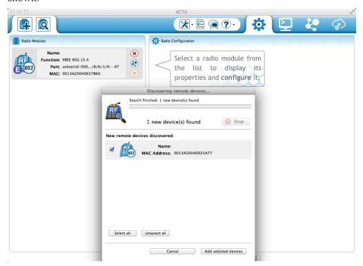
3) You should now see your remote device listed under the remote modules section under your local XBee (the one connected to your computer). The function shows as "Could not initialize device" because it is not connected to the computer for configuration.
