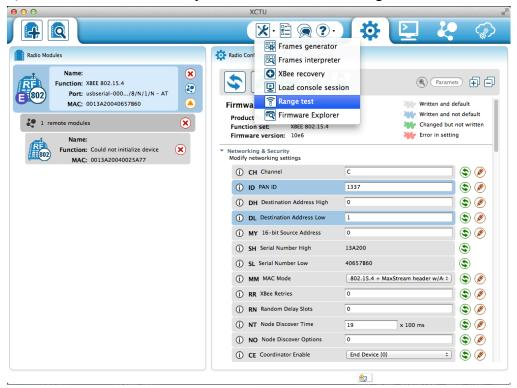
5) A new window will pop up for the range test. Click on your local device on the left section and then select the remote device on the right section. Click on Start Range Test begin.
