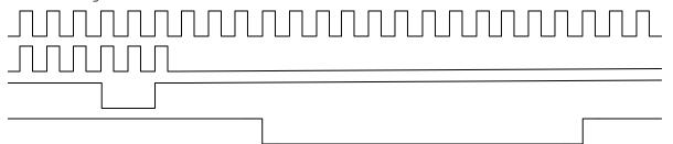
There is clearly a large variability in the timing of valid signal output by a single 6 pulse burst from an infrared transmitter. This is clearly why infrared used by television remotes is such a slow communication medium.
