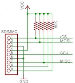
Remark: this schematic includes pull-up's to  $3.3\mathrm{V}$ , which can be left off.
