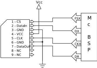
The frame sync from the McBSP port is used to select the card whenever a databyte has to be transferred, it is connected to the chip select of the SD card. The DX and DR pins are connected to the SDcard's DataIn and DataOut lines respectively. Finally the McBSP will have to generate a clock for the SDcard so that it can perform operations, this is accomplished by connecting the clock transmit line of the McBSP port to the CLK pin of the SDCard.
