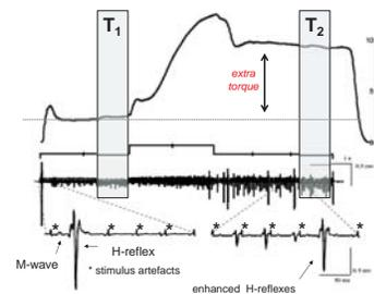
Figure 2. Data analysis. Torque and soleus EMG were quantified before (T<sub>1</sub>; 2-3s into the stimulation) and after (T<sub>2</sub>; 6-7s into the stimulation) 100 Hz stimulation. M-waves and H-reflexes were measured peak to peak and reported as % M<sub>max</sub>. Torque is expressed as % of increase from T<sub>1</sub> to T<sub>2</sub>. (Adapted from Klakowicz et al.<sup>3</sup>)
