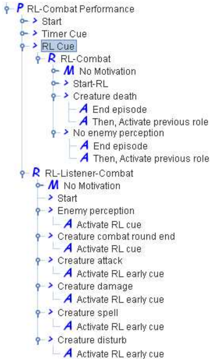
Figure 4.13: The Activate RL cue action starts a generic RL step, the Activate RL early cue action starts an early RL combat step, and the End episode action ends a generic RL episode.
