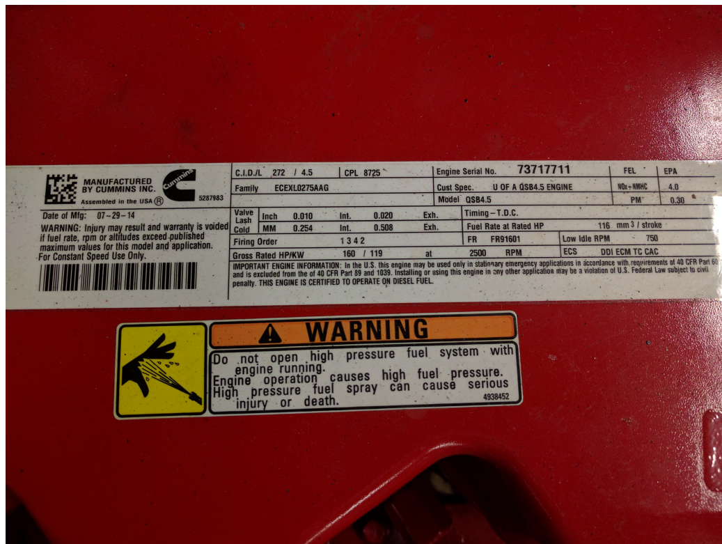
Figure 2.2: Engine Nameplate Showing Model and Serial Numbers, and Nominal Rated Power
