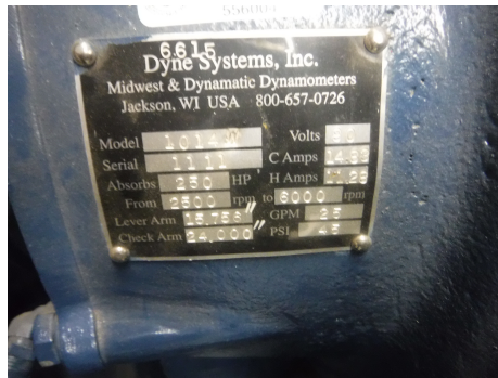
Figure 2.6: Nameplate of Dynamometer Used to Load Engine For Testing
