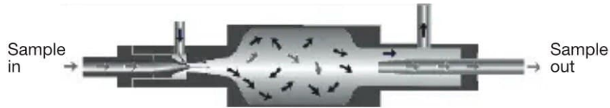
Figure 3.6: Dekati DI-1000 dilutor schematic [2]
