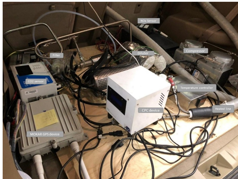
Figure 3.2: A picture of experimental setup inside 2008 Toyota highlander car
