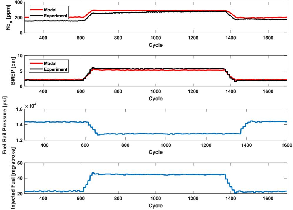
Fig. 3:  $\text{NO}_x$  and BMEP transient response of the engine control oriented model compared to measurement for input of injected fuel amount and rail pressure and measured  $\text{NO}_x$  and BMEP. Engine speed = 1500 rpm
