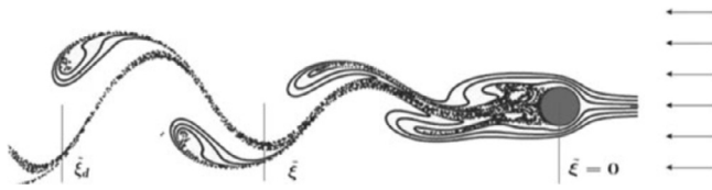
Fig. 1. Vortex shedding in the 2D flow behind a cylinder [1].
