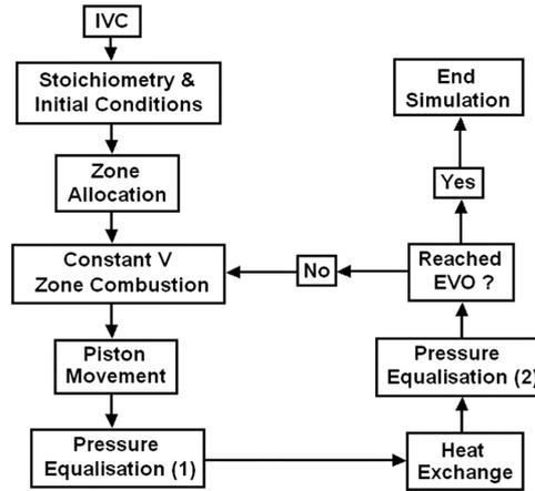
First, each zone is treated as an independent, homogeneous, constant volume reactor. There is no diffusion, mixing, heat transfer, volume change or even mass transfer between zones during this process. Given these conditions, the energy and species conservation equations at constant volume are solved simultaneously for each zone (Kee et al., 2000):
