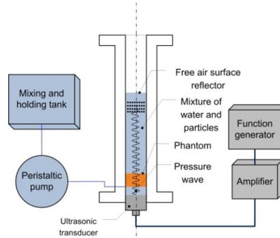
**Figure 1.** Schematic of the experimental system
