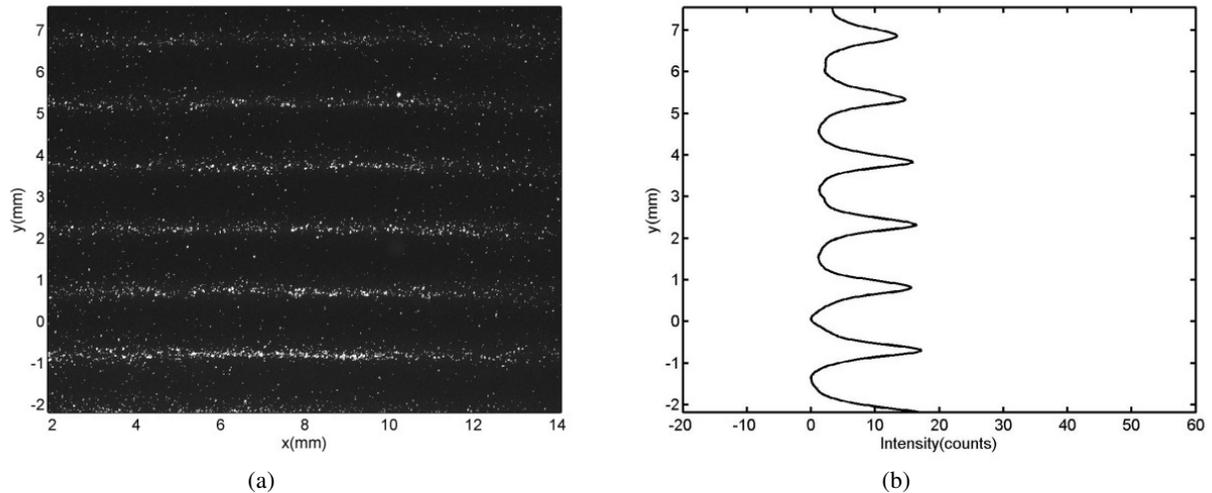
**FIGURE 2.** (a) Formation of particles to the bands and (b) Summed intensity of image in (a) in  $x$  direction
