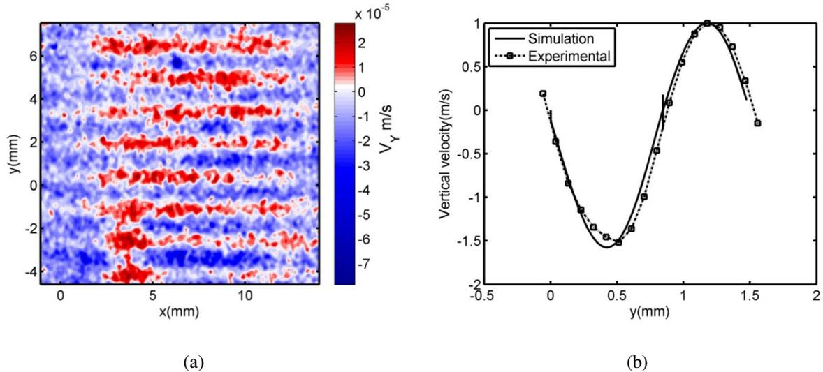
**FIGURE 3.**(a)Vertical velocity contour of particles while formation of bands, (b)Experimental and simulation velocity comparison of banding of particles
