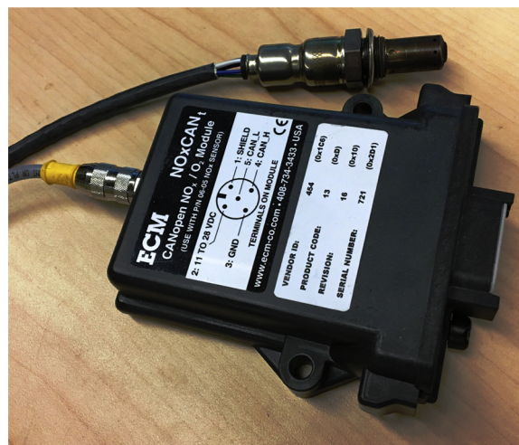
Fig. 1. ECM production \text{NO}_x sensor and the corresponding control module.
