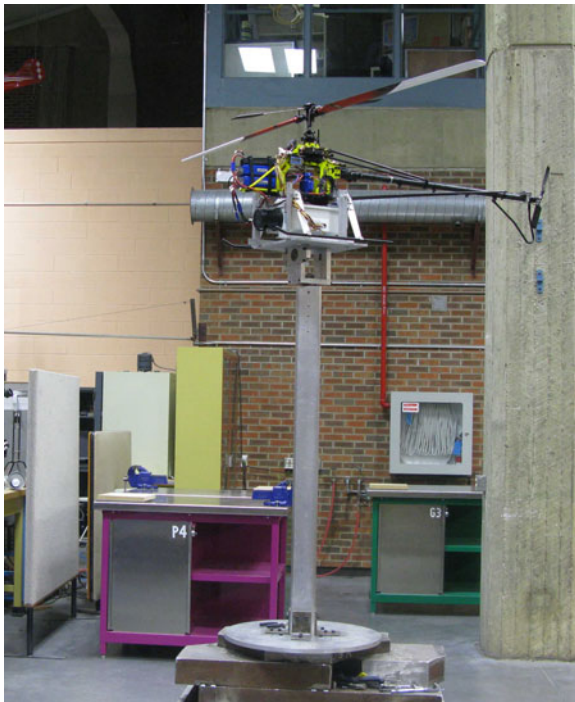
Fig. 23 HIL testbed setup for the heading control
