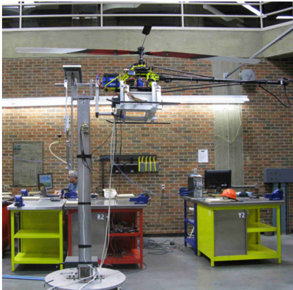
Fig. 16 HIL testbed setup for the lateral control in hover
