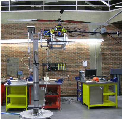
Fig. 11. HIL testbed setup for the roll control in hover
