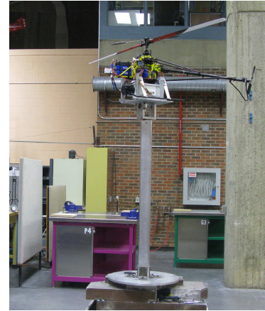
Fig. 14. HIL testbed setup for the yaw control
