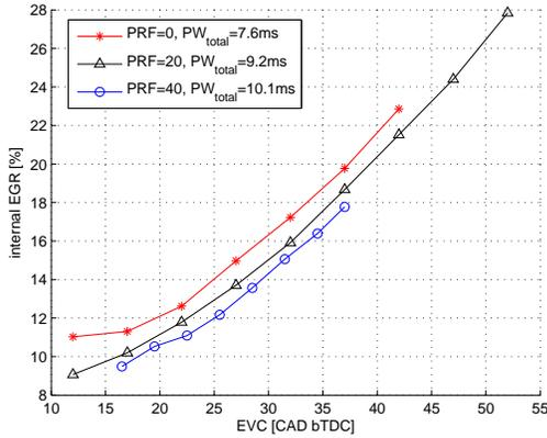
Figure 3: Estimated internal EGR for the exhaust valve timing ranges.
