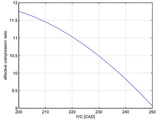
Figure 4: Effective compression ratio for the intake valve timing ranges.
