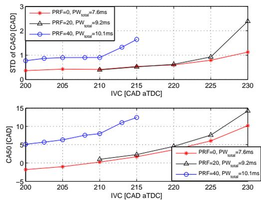
Figure 8: Influence of the timing of the intake valve on cyclic variation of CA50.
