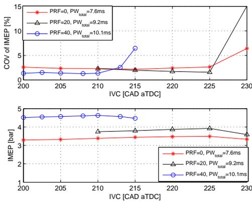
Figure 7: Influence of the timing of the intake valve on cyclic variation of IMEP.
