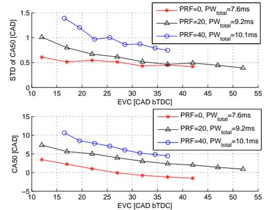
Figure 6: Influence of the timing of the exhaust valve on cyclic variation of CA50.
