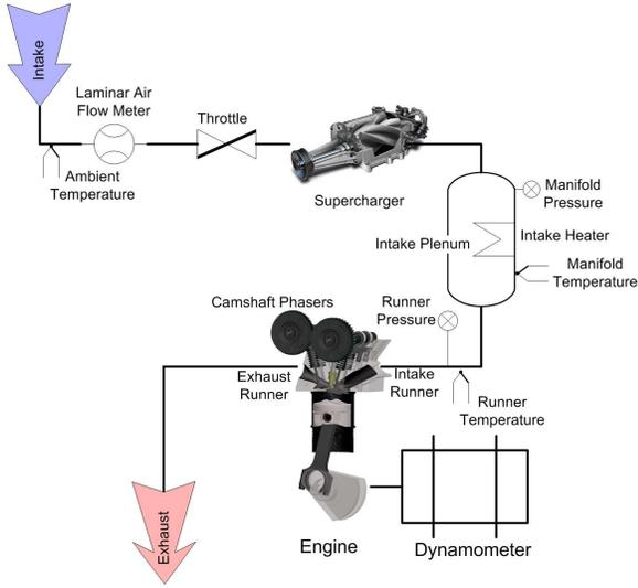
Figure 1: HCCI engine with camshaft phasing cylinder head.
