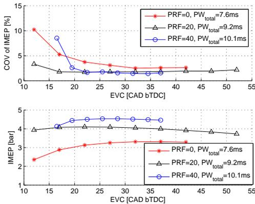
Figure 5: Influence of the timing of the exhaust valve on cyclic variation of IMEP.
