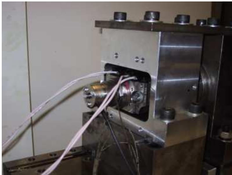
Figure 5.14: LVDT sensor placed in the front of the actuator housing.
