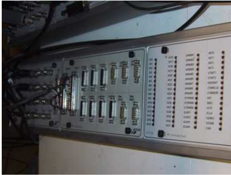
Figure 5.5: DS1103 board expansion box: i/o ports and LED panels.
