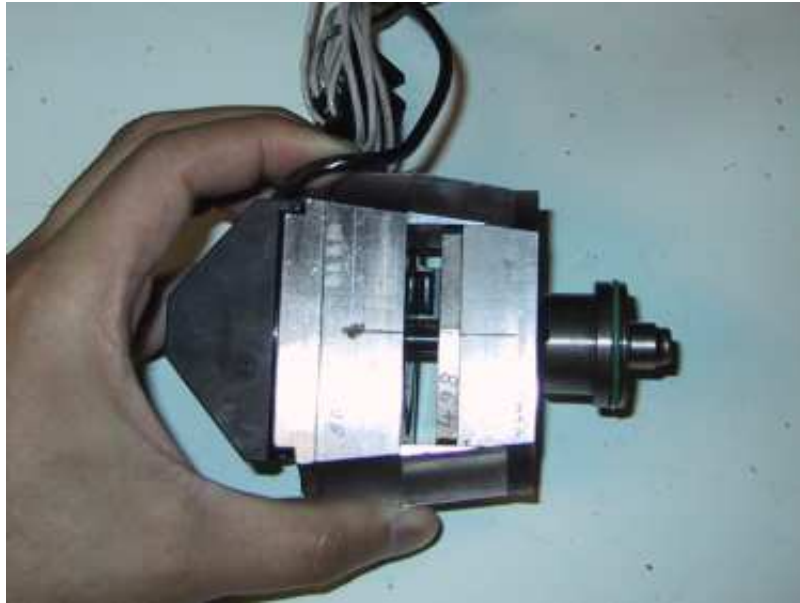
Figure 5.2: Closeup of the EMV actuator (without the springs).
