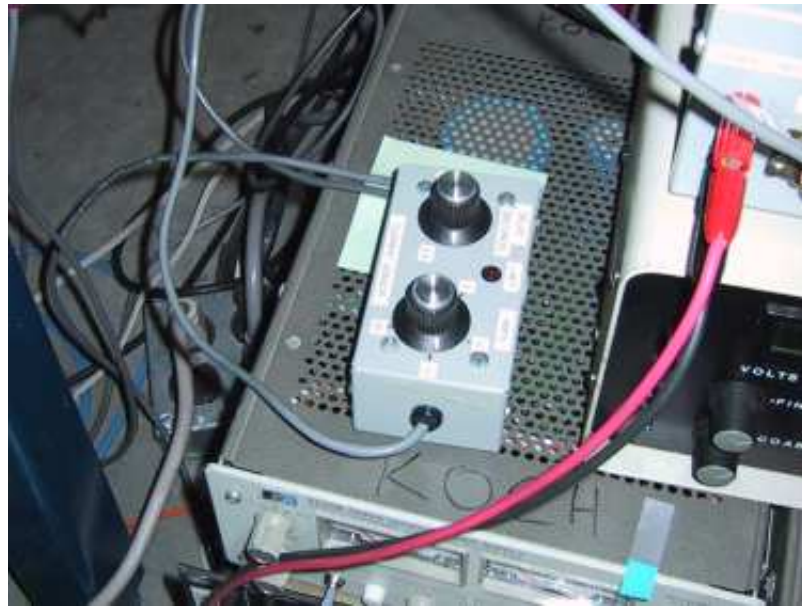
Figure 5.11: Over-current protection device (center).
