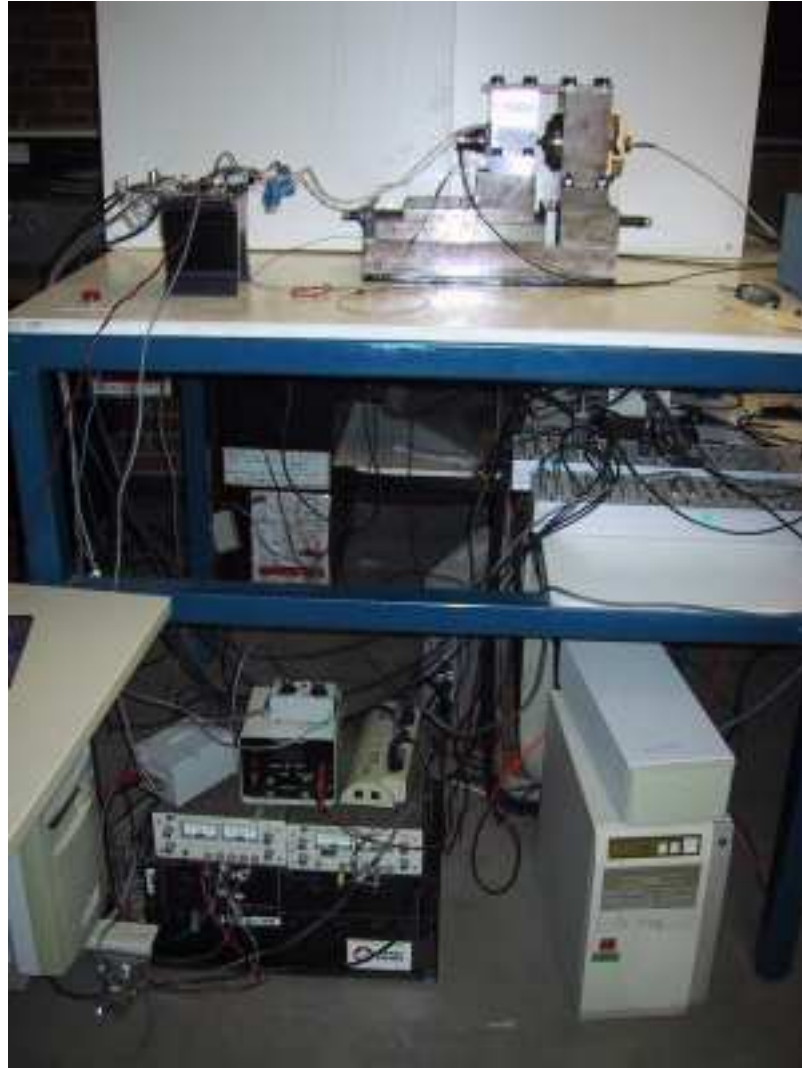
Figure 5.1: Complete actuator test-bench setup, including power supplies and power electronics.
