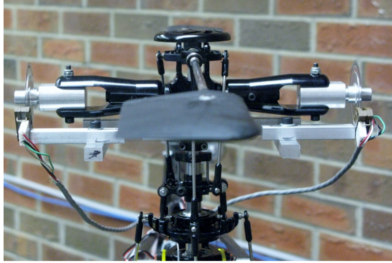
Figure 4.6: The measurement setup for the main rotor mechanism.
