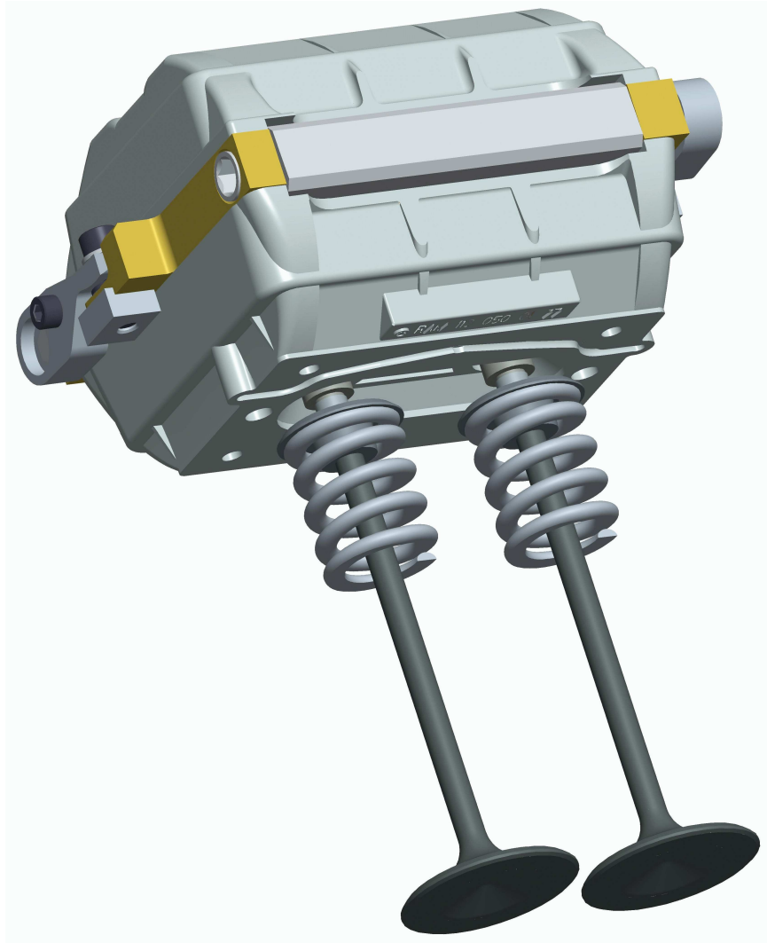
Figure 4.1: 3D solid model of the prototype actuator
