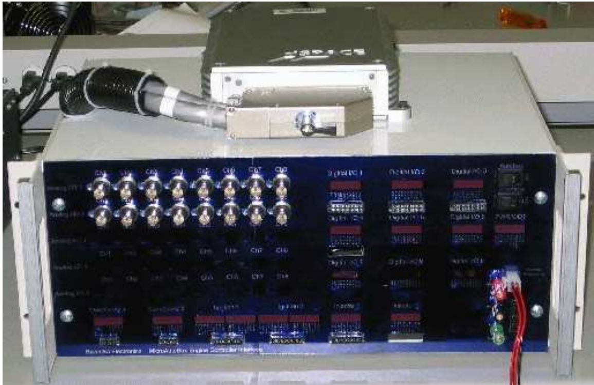
Figure 6.7: dSPACE MicroAutobox and custom interface electronics
