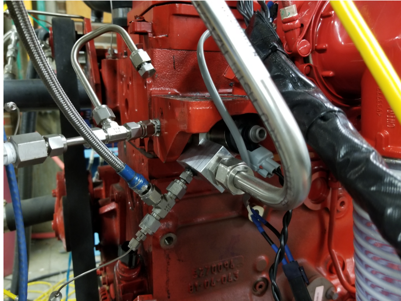
Figure 3.3: Image of the populated holes bored into the head for intake port temperature monitoring and hydrogen injector installation with mounted items.
