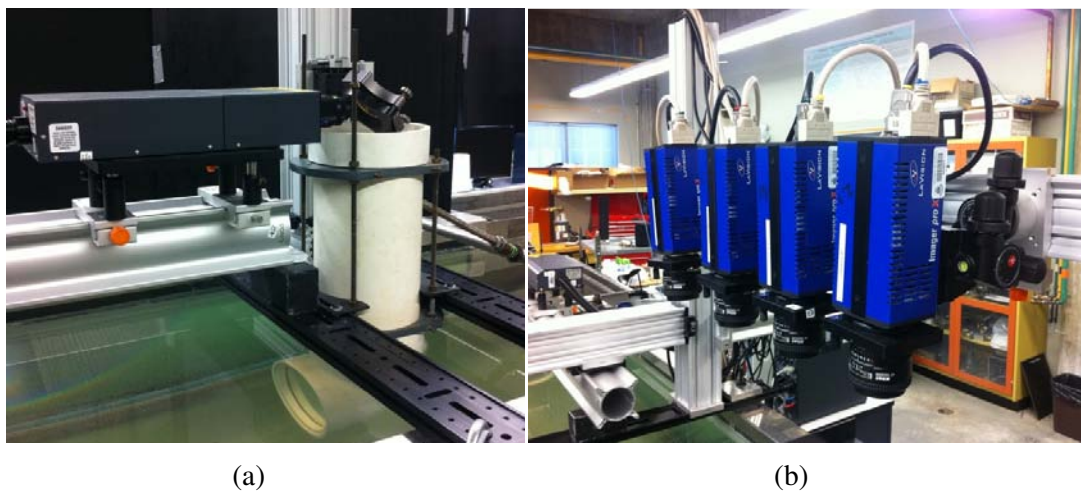
Figure 2.11: a) laser mounting and b) 4 CCD cameras
