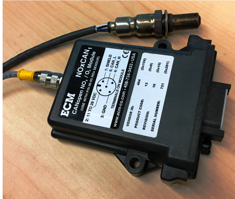
Figure 3.1: ECM production NO x sensor and the corresponding control module
