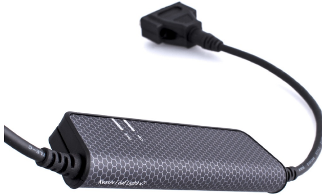
Figure 3.3: Kvaser Light HS CAN interface
