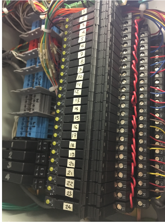
Figure 3.16: Solid state relays for test rig actuators. Pin layout is available in Appendix C.
