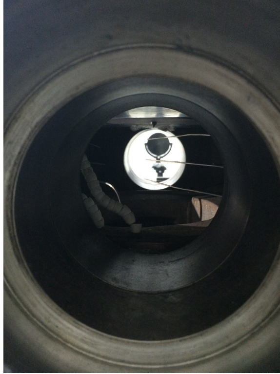
Figure 3.3: Temperature calibration image showing thermocouple positions.
