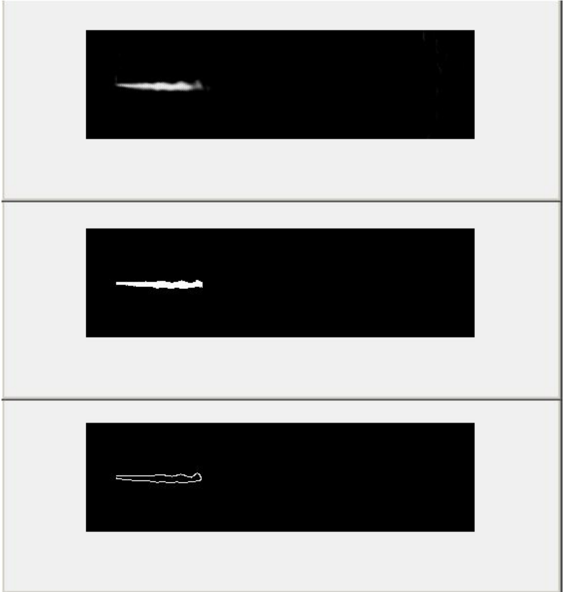
Figure 3.8: Sample image of processing liquid jet (top to bottom: subtracted Image, detected Contour, Canny edge detection contour).
