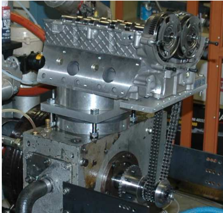
Figure B.3: The timing chain and gear set that drive that camshafts. This figure also shows the impulse wheel for the hall effect sensor.
