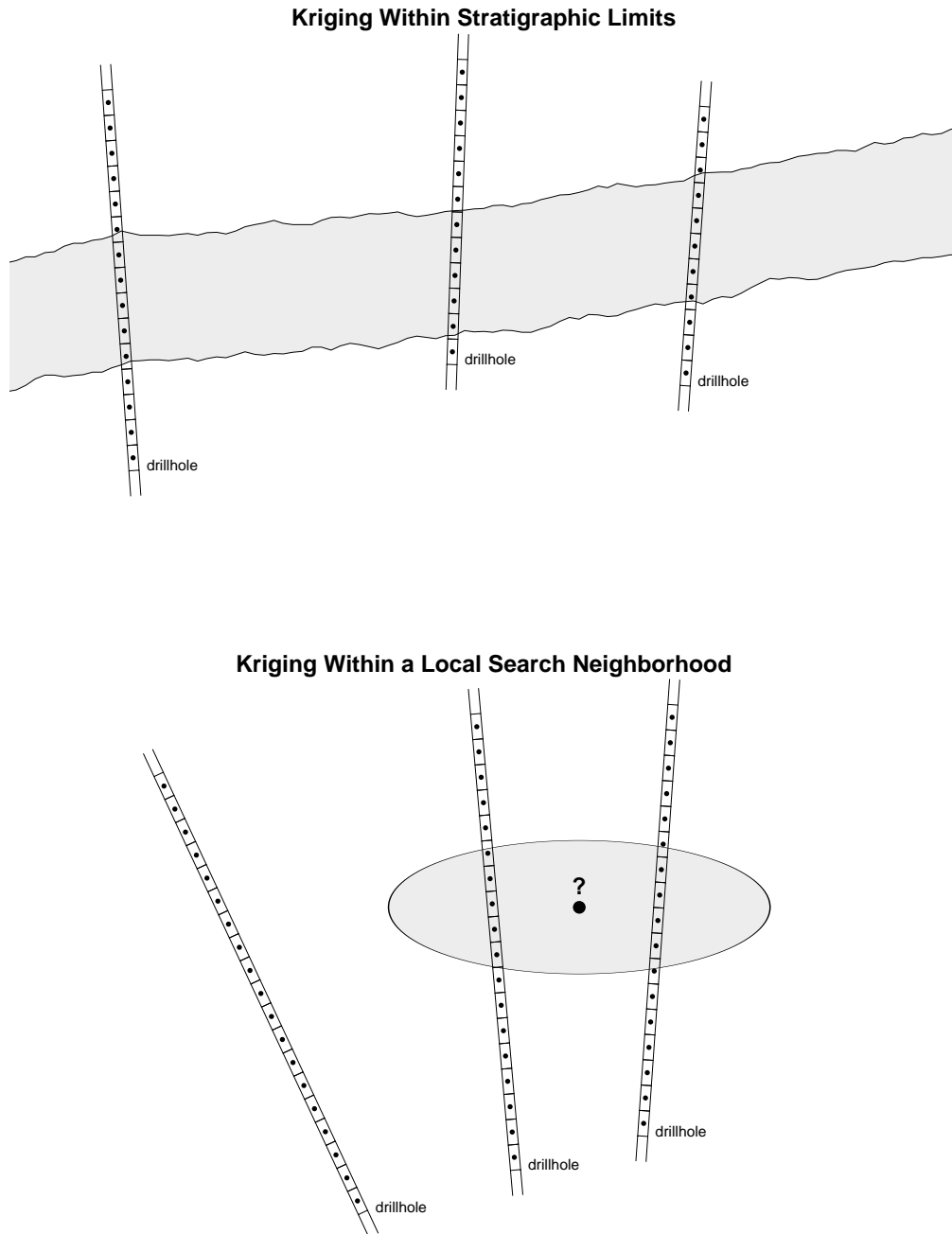
Figure D.1: Two commonly encountered situations when finite strings of contiguously aligned data are used in kriging. In the top figure the shaded area represents a stratigraphic layer of interest. The shaded area in the bottom figure represents the limits of a local search neighborhood.
