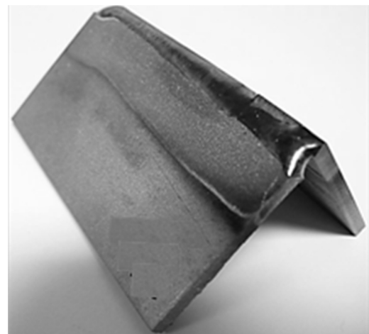
Fig. 3. Example of complete total longitudinal welding of Ti6Al4V alloy in flush corner joint configuration. (Tracking speed = 0.15 m/s; Solar insolation = 1000 W/m 2 ).
