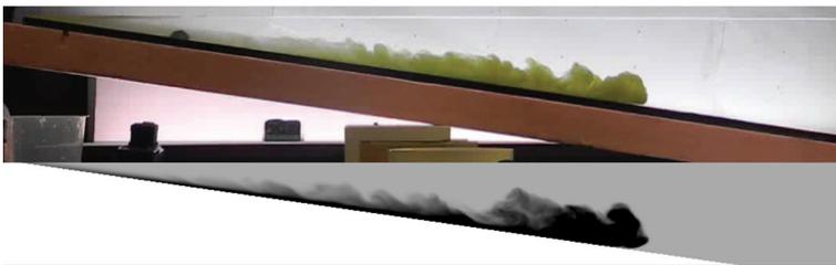
**Fig. 3** Snapshots of a turbidity current experiment (exp2, based on experiments by Snow and Sutherland [23],  $S = 0.176$ ,  $Re = 15,000$ ,  $\nu_s = 0.001$ ,  $m = 0.149$ ) right before separation of the current from the bottom slope. Experimental results (top) and the corresponding numerical results are compared at time  $t = 12.1$
